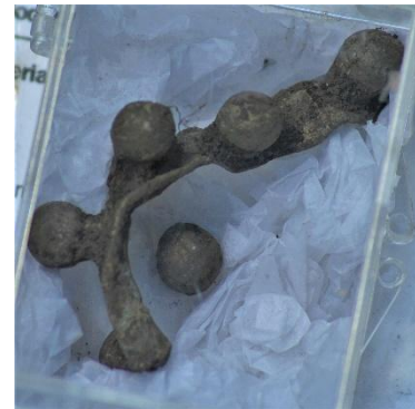
A casting sprue – shot towers had not yet been created, although the idea of dropping shot to make it round was known.
